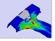
Accuracy of forming simulations strongly depends on the consideration of temperature dependent viscoplasticity
